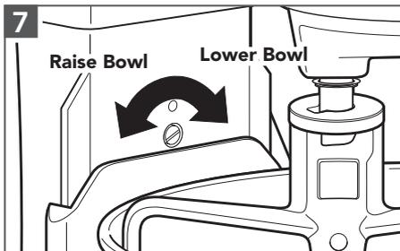
**7** **(OPTIONAL) To adjust Beater to Bowl clearance:** Lower the Bowl to the down position. Turn the screw slightly counterclockwise (left) to raise the Beater, or clockwise (right) to lower it. Adjust the beater so that it just clears the surface of the Bowl. Check again the clearance of the Beater to the Bowl.
