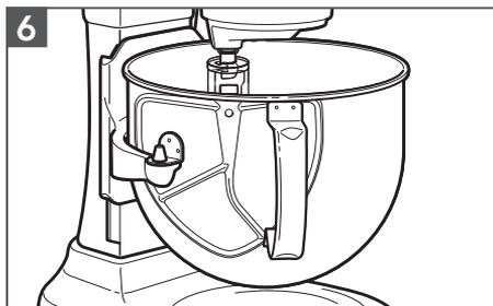
**6** **Test the beater to bowl clearance:** Plug the Stand Mixer into an earthed outlet. Turn Stand Mixer ON and test each speed, making sure the beater does not touch the bowl during operation. If the beater is too far away from the bottom or is hitting the Bowl, proceed to next step to make adjustments.
