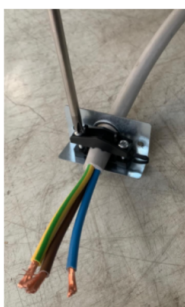
Fix power cord to the plastic holder.
