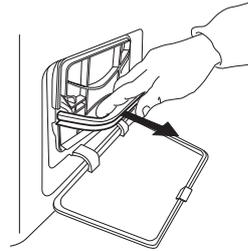
Open the bottom flap. Hold the handle and pull out the bottom filter.
