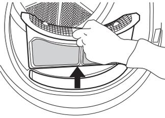
Press the button to open the door filter. Remove the lint inside. Close the filter and reinsert it in the right direction, so that it completely integrates in the filter chamber.
