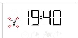
Please note: During cooking you can change the function by turning the selection knob or adjust the temperature by turning the thermostat knob. The function will not start if the thermostat knob will be on **0 / AUTO** position. You can set the cooking time, cooking end time (only if you set a cooking time) and a timer.
