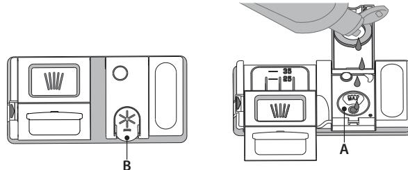
1. Open the dispenser **B** by pressing and pulling up the tab on the lid.
