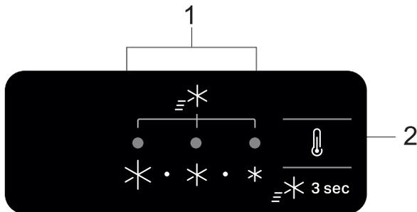
1. Indicator Leds (to display the current temperature set point or the Fast Cooling function)
