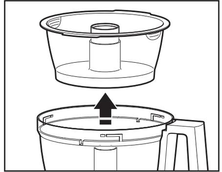
6. Turn the work bowl to the left to unlock it from the base. Lift to remove.
