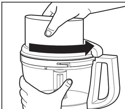
2. Fit the food pusher into the 3-in-1 feed tube. See "Using the 3-in-1 Feed Tube" for details on working with different sized foods.
