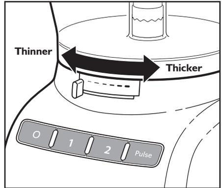
**NOTE:** The lever only works with the adjustable slicing disc. Changing thickness settings with other discs or blades installed will have no effect on operation.
