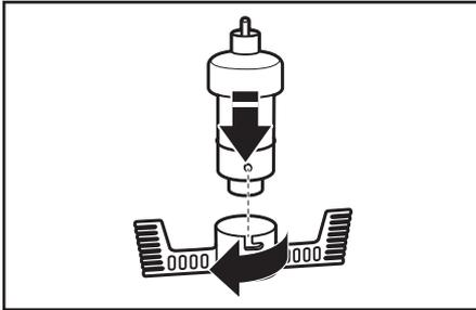
2. With the work bowl in place on the base, place the egg whip on the power shaft.
