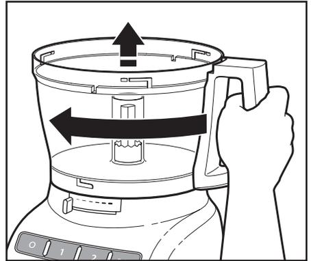
7. The multipurpose blade can be removed from the work bowl before the contents are emptied. You may also leave the blade locked in place. Then remove food from the bowl and blade with a spatula.
