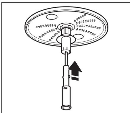
3. With the work bowl installed, slide the drive adapter onto the power shaft.
