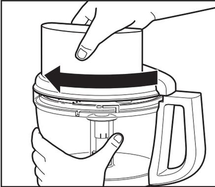
4. If using a disc, remove it before removing the bowl. Holding the disc by the 2 finger grips, lift it straight up. Remove the adapter.
