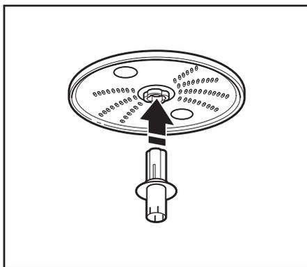
2. Slide the drive adapter into the disc adapter as far as it will go, until it clicks into place.
