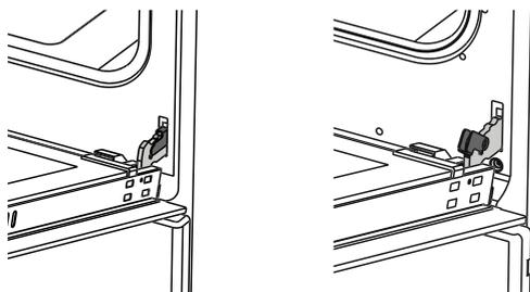
Later, close the opened oven door so that it will be in a position to contact with hinge lock.
