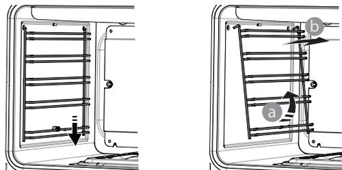
To refit the grilles, insert the top support, then slide them to be fitted close to the cavity and push them up to fix in their original position.
