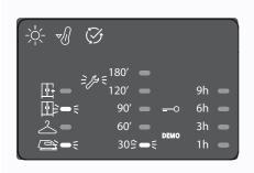
The presence of wrench symbol signals a malfunction. Carry out the operations described. Switch the dryer off and unplug it. Open the door immediately and pull landry out, to allow the heat to dissipate. Wait for about one hour. Reconnect the dryer to the power supply, load the laundry and restart the drying cycle.
