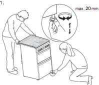
**CAUTION:** Some soft floor coverings may get damaged if the cooker is not moved carefully. Badly leveled device may increase condensation. **NOTE:** Ensure oven shelves are level by using a spirit level on the rod shelves.
