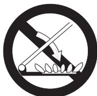
WARNING! The glass lid can break in if it is heated up. Turn off all the burners and the electric plates before closing the lid.
