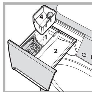
This function is particularly useful for the removal of stubborn stains. Insert extra compartment 4 (supplied with the appliance) into compartment 1. When pouring in the bleach, be careful not to exceed the "max" level marked on the central pivot (see figure). To bleach laundry with no other washing action, pour the bleach into extra compartment 4, select the "Rinse" cycle and activate the "Stain
