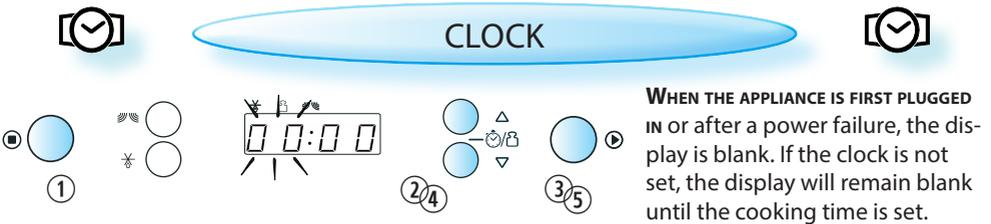
**WHEN THE APPLIANCE IS FIRST PLUGGED IN** or after a power failure, the display is blank. If the clock is not set, the display will remain blank until the cooking time is set.
