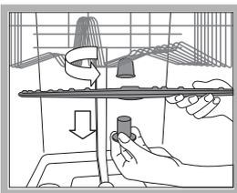
To remove the upper sprayer arm, rotate the locking ring in an anti-clockwise direction. The upper sprayer arm should be replaced with the holes facing upwards.
