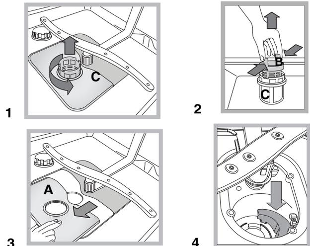
After cleaning the filters, replace the filter assembly and fix it in position correctly; this is essential for maintaining the efficient operation of the dishwasher.
