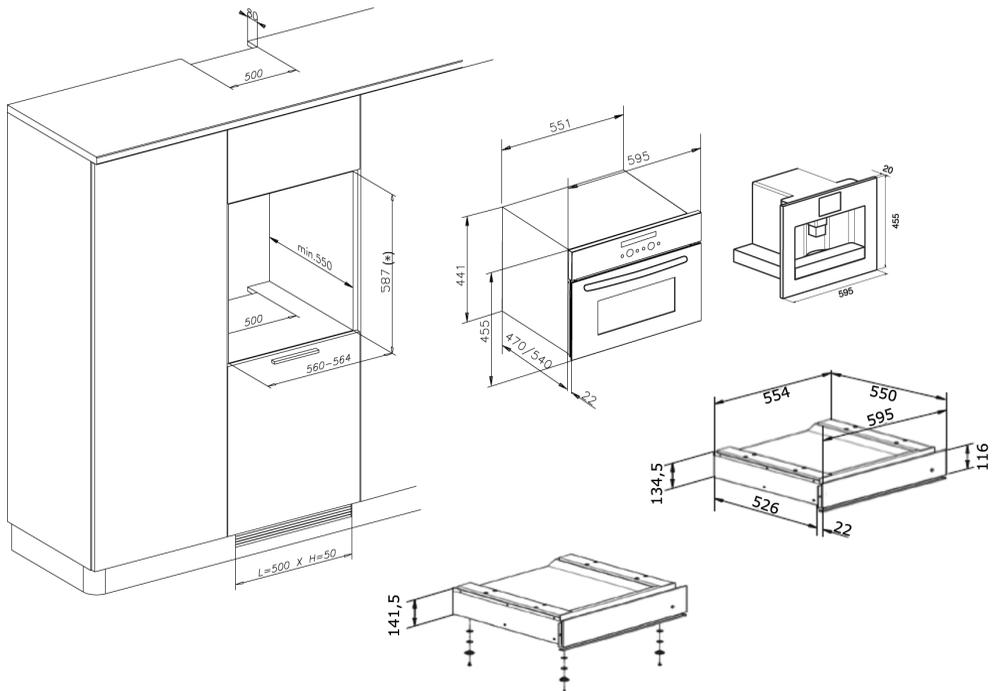
(\* ) In case of 595 cabinet recess height, the drawer must be installed with the 4 feet and respective 1 mm washers (included in the packaging) in the lower part.
