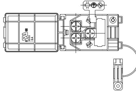
The appliance must be connected to the electricity supply by means of an all-pole disconnect switch with minimum contact gap of 3 mm.
