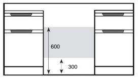
Gas hose connection point must be installed within the shaded area
