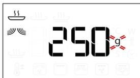
When the default setting appears on the display and the
