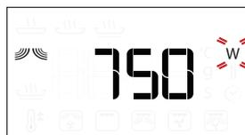
When the **W** icon flashes on the display, turn the *knob* to adjust the power setting and then press
