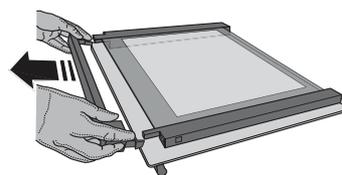
**2.** Lift and firmly hold the inner glass with both hands, remove it and place it on a soft surface before cleaning it.
