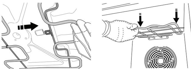
**2.** To return the heating element to its position, lift it up, pull it slightly towards you and make sure that the tab support is in its proper seating.
