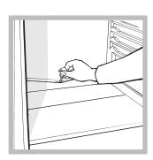
special discharge outlet (see diagram) where the heat produced by the compressor causes it to evaporate. It is necessary to clean the discharge hole regularly so that the water can flow out easily.
