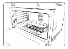
Remove the screw securing the oven burner and withdraw the burner from the support together with the heat sensor and the ignition spark plug.
