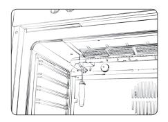
Remove the injector using the 7 mm socket wrench.
