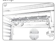
Remove the burner together with its heat elements.
