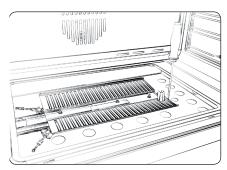
Remove the nozzle using a 7 mm socket wrench.
