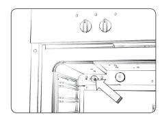
Fully tighten the new injector which must be of the diameter indicated in the table in the chart table.
