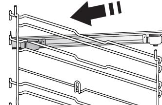
Fasten the upper clip of the runner to the shelf guide and slide it along as far as it will go. Lower the other clip into position.
