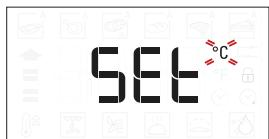
Turn the selection knob to select the unit of measurement, then press **OK** to confirm.
