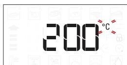
When the °C/°F icon flashes on the display, turn the knob to change the value, then press
