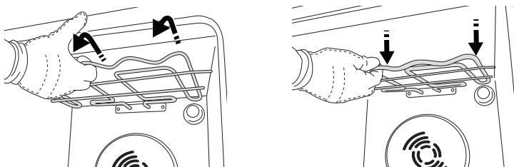
3. To reposition the heating element, lift it up, pulling it slightly towards you, making sure it comes to rest on the lateral supports.
