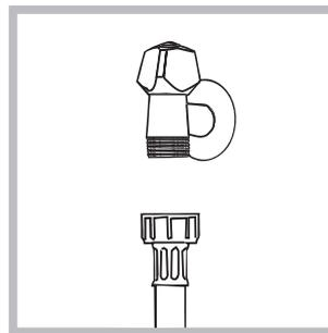
1. Connect the inlet hose by screwing it to a cold water tap using a 3/4 threaded connection (see figure). Before performing the connection, allow the water to run freely until it is perfectly clear.
