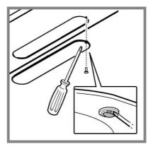
Replace the damaged lamp.
