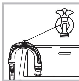
Alternatively, place the drain hose over the edge of a washbasin or bathtub, by fastening the guide (which can be purchased at the technical assistance centre) to the tap (see figure). The free end of the hose
