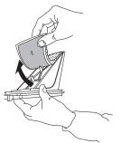
Fix the filter foam on the bottom filter. Clean the filter chamber of the dryer with a damp cloth or carefully with a vacuum cleaner. Insert the bottom filter again. Clap the filter handle down and close the bottom flap.
