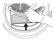
Press the button to open the door filter. Remove the lint inside. Close the filter and reinsert it in the right direction, so that it completely integrates in the filter chamber.
