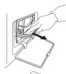
Open the bottom flap. Hold the handle and pull out the bottom filter.
