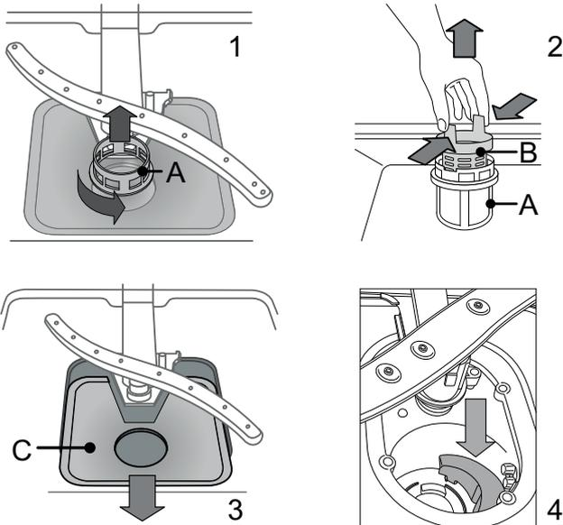
After cleaning the filters, re-place the filter assembly and fix it in position correctly; this is essential for maintaining the efficient operation of the dishwasher.
