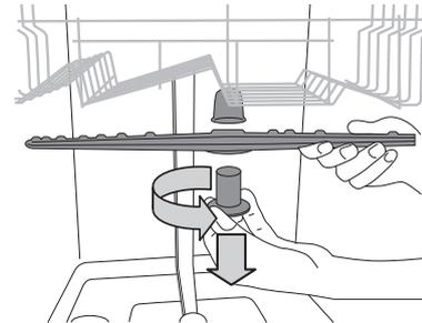
To remove the upper spray arm, turn the plastic locking ring in an anti-clockwise direction. The upper spray arm should be replaced so that the side with the greater number of holes is facing upwards.
