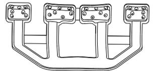
The lower rack has a Space Zone, a special pull-out support in the rear of the rack that can be used to support frying pans or baking pans in upright position, thus taking up less space.
