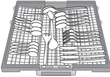
The third rack was designed to house the cutlery. Arrange the cutlery as shown in the figure. A separate arrangement of the cutlery makes collection easier after washing and improves washing and drying performance.
