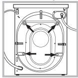
3. Remove the 4 protective screws (used during transportation) and the rubber washer with the corresponding spacer, located on the rear part of the appliance (see figure).
