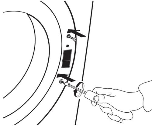
**20.** Fix the door on the left side of the door opening by turning in the two screws.
