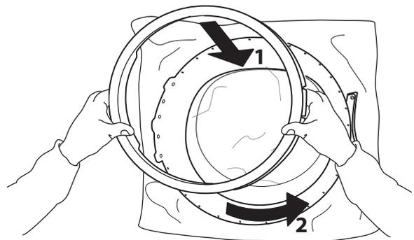
**17.** Turn the door again and lay it upside down. Fix the bottom screw again.
