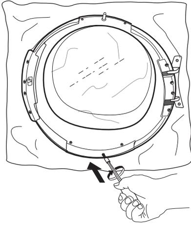
**18.** Insert the door lock on the right side of the door opening. Press it completely inside the hole and move it a bit downwards, until the small knob of the door lock latches.
