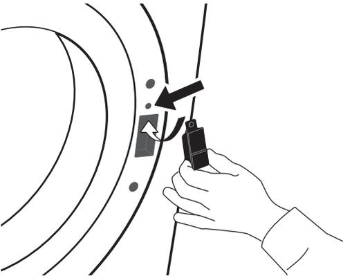
**19.** Fix the two screws over and under the door lock, on the right side of the door opening.
