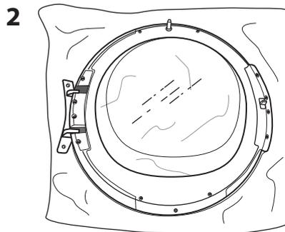
**9.** Remove the two side screws. Do this on both sides of the door.
