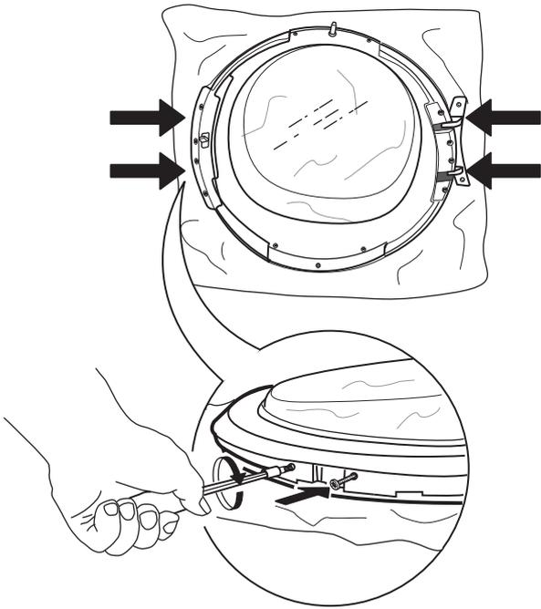
**15.** Turn the door and lay it down on the door glass.
