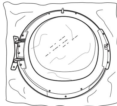
**5.** Unscrew the bottom screw, to release the cover frame on the front of the door.
