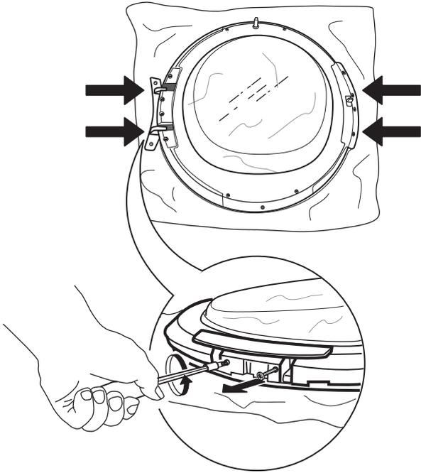
**10.** Remove the 4 inner screws on each side of the door.
