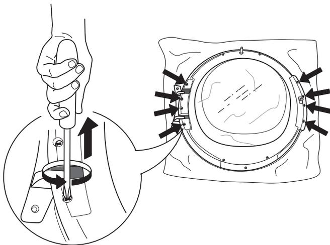
**11.** Remove the side parts on each side of the door.
