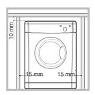
Install the dryer far from gas ranges, stoves, radiators or hobs as flames may damage it. If the dryer is installed below a worktop, ensure there are 10 mm between the upper panel of the dryer and any objects above it and 15 mm between the sides of the machine and the walls or
