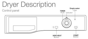
The HEAT button selects drying temperature.
