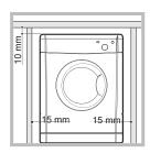
If you are going to install the appliance under a work counter be sure to leave a 10mm space between the top and any other objects on or above the machine and a 15mm space between the sides and any kitchen units or walls to ensure proper air circulation. The
