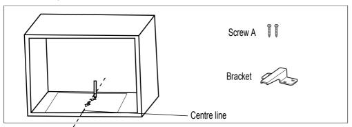
3. Remove the bottom cabinet template and fix the bracket with screw A.
