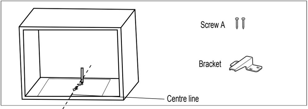
3. Remove the bottom cabinet template and fix the bracket with screw A.
