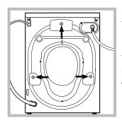
3. Remove the **3** protective screws and the rubber bush with the respective spacer, situated on the rear of the appliance (see also the installation leaflet).
