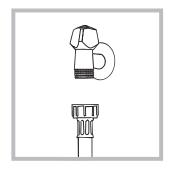
2. Connect the inlet hose by screwing it to a cold water tap using a 3/4 threaded connection (see figure).
