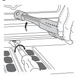
6. Replace all the parts, following the steps described above in the reverse order. Take care to replace also the bottomof the oven in its original position.
