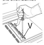
5. Unscrew the oven burner nozzle using the special socket spanner for the nozzles, or better still a 7 mm socket spanner, and replace it with a nozzle suited to the new type of gas (see Table 1).
