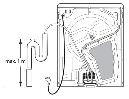
**NOTE:** To avoid siphoning, the end of the hose must not be immersed in the drain water. Avoid bending and twisting the hose.
