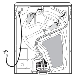
**C.** Fix the hose to the sewage system. The height difference between the floor where the dryer stands on and the connection at the sewage system should not exceed 1 m.
