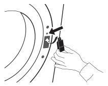
**7.** Fix the 2 screws above and below the door lock system.
