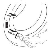
For removing and fixing the door, the help of a second person is recommended. Make sure that the dryer is unplugged. Open the dryer door.
