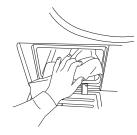
**7.** Push the bottom filter back into the filter compartment; make sure that it is completely integrated. Turn both locking bars (right and left) back into vertical position, to lock the bottom filter.
