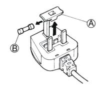
1. Remove the fuse cover (A) and fuse(B).
