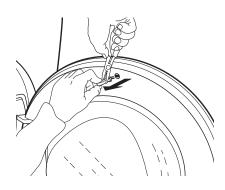
**2.** Unscrew the 2 screws above and below the door lock system.
