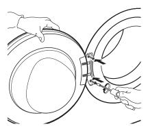
**6**. Insert the door lock on the right side of the door opening. Press it completely inside the hole and move it a bit downwards, until the small knob of the door lock latches.
