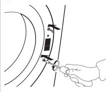
8. Insert the contact pin on top inside of the door. Turn the contact pin with pliers by 90° towards the right, to lock it.
