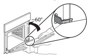
**4.** Take a firm hold of the door with both hands – do not hold it by the handle. Simply remove the door by continuing to close it
