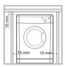
If you are going to install the appliance under a work counter be sure to leave a 10mm space between the top and any other objects on or above the machine and a 15mm space between the sides and any kitchen units or walls to ensure proper air circulation.
