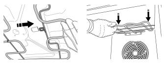
**2.** To reposition the heating element, lift it up and pull it slightly towards you, making sure to fit it into its seating.
