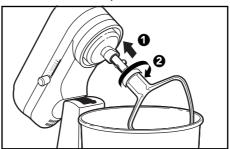
5. Unlock the Motor Head and move it down. Then, lock\*\* the head to keep it down. Before mixing, test lock\*\* by attempting to raise the Motor Head.
