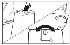
**NOTE:** When properly adjusted, the Flat Beater will not strike on the bottom or side of the Bowl. If the Flat Beater or the Wire Whip is so close that it strikes the bottom of the Bowl, the beater or whip may wear.
