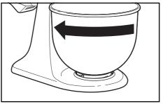
**4.** With the Motor Head lifted and locked, slide the accessory over the shaft, aligning with the pin, then rotate clockwise to hook it over the pin on the shaft.
