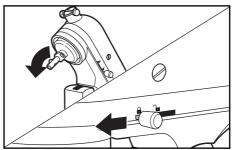
**(OPTIONAL) To Adjust Beater to Bowl Clearance:** Tilt and lock\*\* the Motor Head back. Locate the screw revealed under the Motor Head. Turn the screw slightly counterclockwise (left) to raise the beater, or clockwise (right) to lower it.
