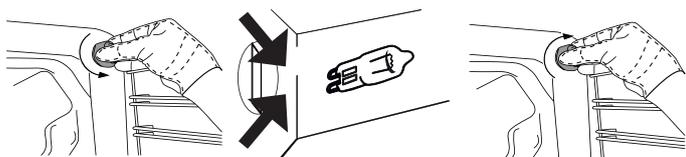
Please note: Only use 15-25 W/220-240 V type G9, T300°C halogen bulbs. The bulb used in the product is specifically designed for domestic appliances and is not suitable for general room lighting within the home (EC Regulation 244/2009).
