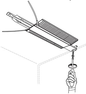
Remove the burner together with its heat elements. Remove the injector using the 7 mm socket wrench.
