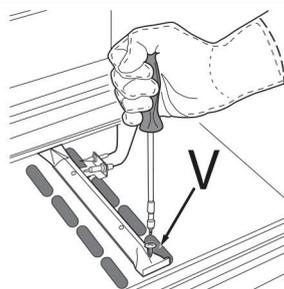
5. Unscrew the oven burner nozzle using the special socket spanner for the nozzles, or better still a 7 mm socket spanner, and replace it with a nozzle suited to the new type of gas (see Table 1).
