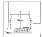
**NOTE:** If the distance "A" between the wall cabinets is between 600 mm and 730 mm, the height "B" must be a minimum of 530 mm. If the distance "A" between the wall cabinets is greater than the width of the hob, the height "B" must be a minimum of 400 mm.
