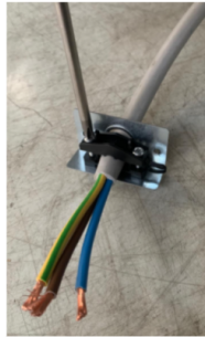
Fix power cord to the plastic holder.
