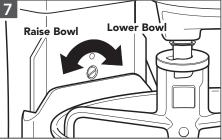
(OPTIONAL) To adjust Beater to Bowl clearance: Lower the Bowl to the down position. Turn the screw slightly counterclockwise (left) to raise the Beater, or clockwise (right) to lower it. Adjust the beater so that it just clears the surface of the Bowl. Check again the clearance of the Beater to the Bowl.
