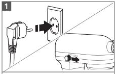
Plug it into an earthed outlet. Start with lower speed to avoid splashing and increase it gradually. Refer to the "Speed Control Guide".
