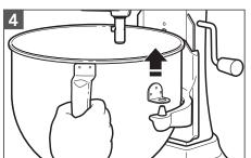
To Remove Bowl: Place Bowl-Lift Lever in the down position. Grasp Bowl Handle and lift straight up and off Locating Pins
