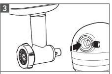
Insert attachment into Attachment Hub, making certain that attachment power shaft fits into the square Attachment Hub socket.
