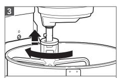
Remove the accessory: Press accessory upward and turn to the left. Pull down the accessory from Beater Shaft.
