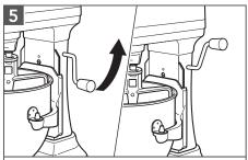
To raise the bowl: Rotate the Bowl-Lift Lever to the straight up position. The Bowl must always be in the raised position when mixing.
