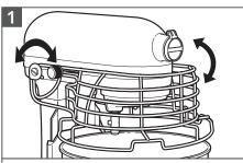
To attach the Bowl Guard\*: Make sure that the guard is returned to the down position before beginning to use the Stand Mixer. The Stand Mixer will not run if the Bowl Guard is not in the proper position.
