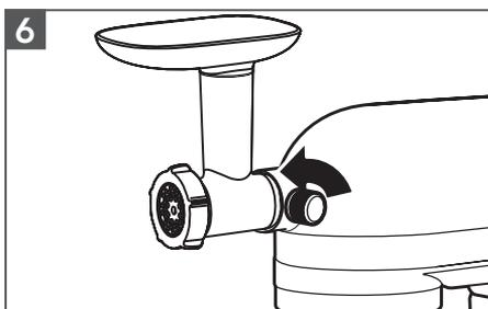
6 Loosen Attachment Knob by turning it counterclockwise. Rotate attachment slightly back and forth while pulling it out.
