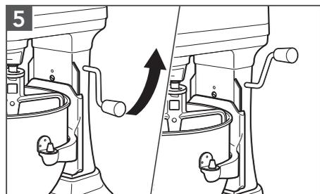
**To raise the bowl:** Rotate the Bowl-Lift Lever to the straight up position. The Bowl must always be in the raised position when mixing.
