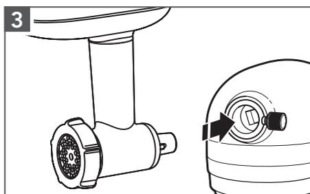
3 Insert attachment into Attachment Hub, making certain that attachment power shaft fits into the square Attachment Hub socket.
