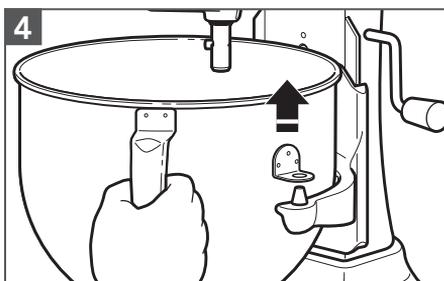
4 **To Remove Bowl:** Place Bowl-Lift Lever in the down position. Grasp Bowl Handle and lift straight up and off Locating Pins
