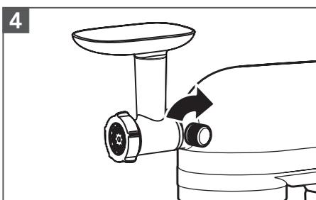
4 Tighten the Attachment Knob by turning it clockwise until the attachment is secured to the Stand Mixer.
