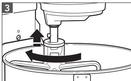
3 **Remove the accessory:** Press accessory upward and turn to the left. Pull down the accessory from Beater Shaft.
