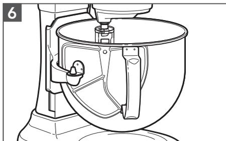
**Test the beater to bowl clearance:** Plug the Stand Mixer into an earthed outlet. Turn Stand Mixer ON and test each speed, making sure the beater does not touch the bowl during operation. If the beater is too far away from the bottom or is hitting the Bowl, proceed to next step to make adjustments.
