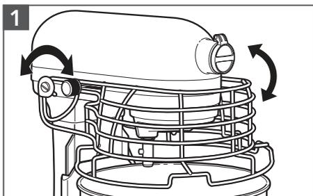
**To attach the Bowl Guard\*:** Make sure that the guard is returned to the down position before beginning to use the Stand Mixer. The Stand Mixer will not run if the Bowl Guard is not in the proper position.
