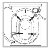
Rémove the 4 protective screws and the rubber bush with the respective spacer, situated on the rear of the appliance (see also the installation leaflet).
