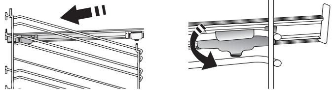
Please note: The sliding runners can be fitted on any level.
