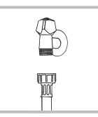
1. Connect the supply pipe by screwing it to a cold water tap using a 3/4 gas threaded connection (see figure). Before performing the connection, allow the water to run freely until it is perfectly clear.
